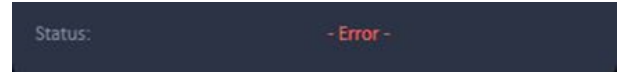
Fig. 150 Definite Focus tool: Find Surface pressed and reflex not found because of insufficient signal strength.
