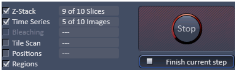
Fig. 77 Multidimensional input field – display of the current status 9 from 10 slices taken from the 5th of the 10 images
