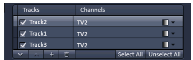
Fig. 129 Track selection display – Track 2 moved to the top, no further upwards movement possible
