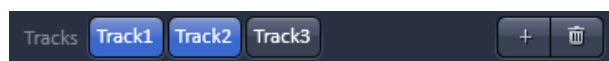
Fig. 127 Imaging Setup tool Tracks display– track selection of track 1 and 2 updated from the Channel tool
